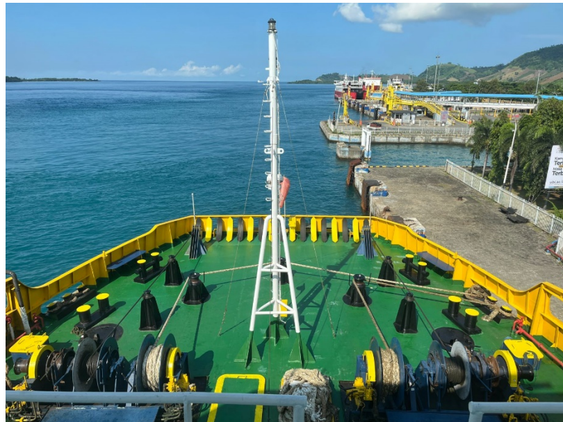
Gambar 2. 3 Layout Tali Haluan KMP. Portlink V
