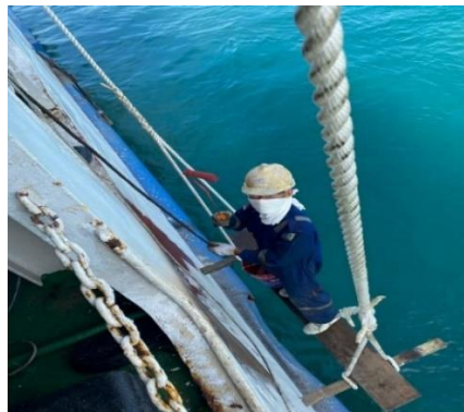
Gambar 4. 9 Painting di lambung kapal tanpa safety harness
