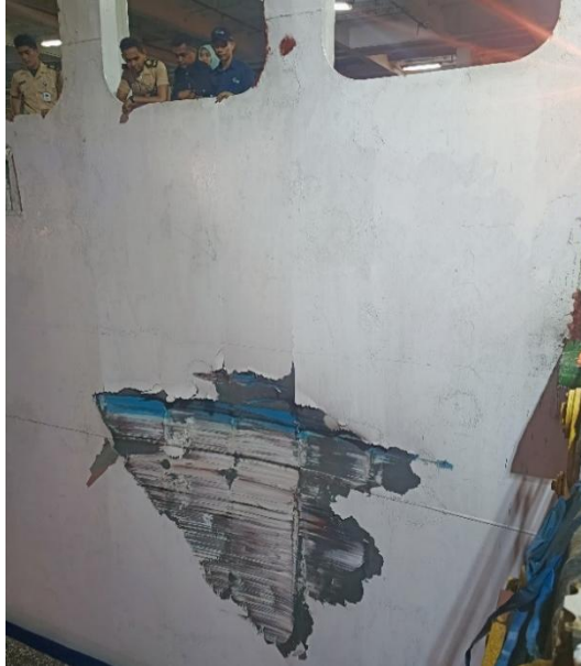
Gambar 4. 4 Pengecekan Plate Lambung Buritan Kiri Kapal
