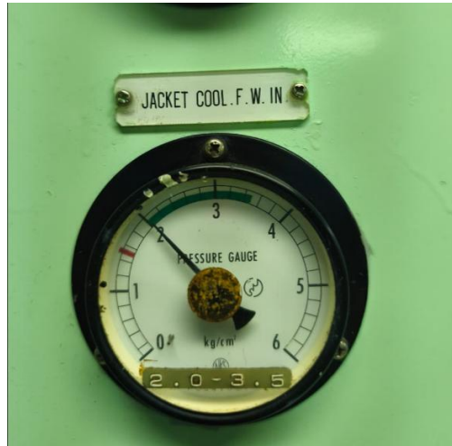
Gambar 4. 5 tekanan pompa air tawar hampir melewati batas normal
