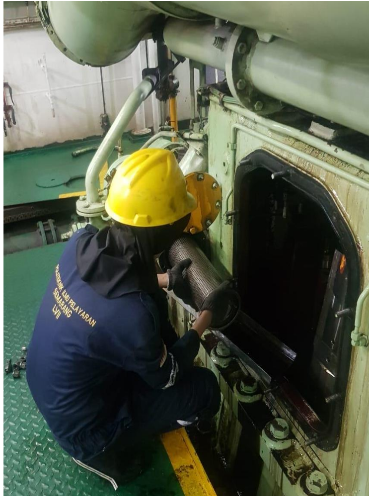
Gambar 4. 12 Pembersihan Filter Strainer
