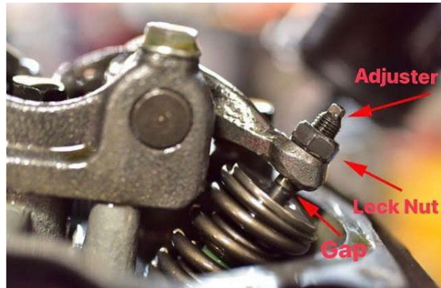
Gambar 2.2. Valve Gap
