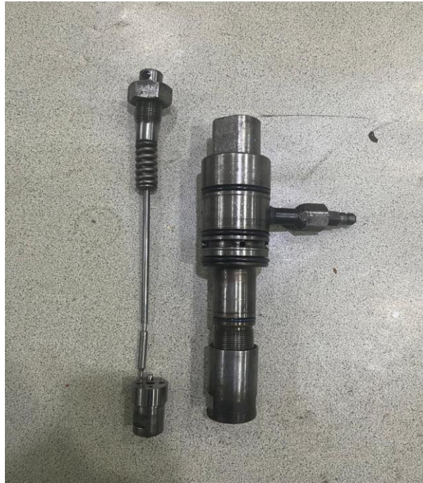
Gambar 2. 2 Injector Diesel Generator KMP. Port Link
