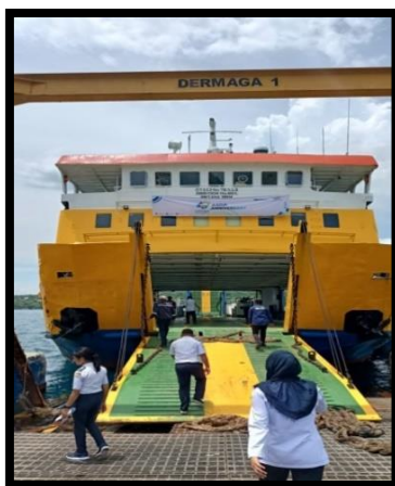
Gambar 4.21 Movable Bridge (MB) I
