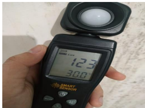
Gambar 4.29 Lux Lampu Penerangan Terminal
