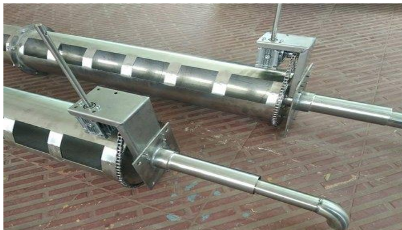
Gambar 2. 2. Slotted Pipe Skimmer
