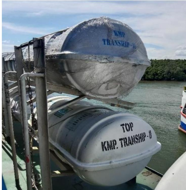
Gambar 4.38 Kondisi Eksisting Liferaft Pada KMP. Tranship II
