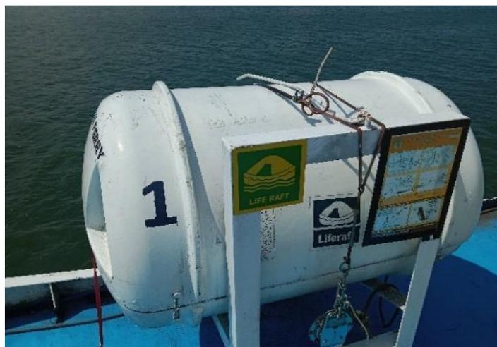
Gambar 4.33 Kondisi Eksisting Liferaft Pada KMP. Ulin Ferry
