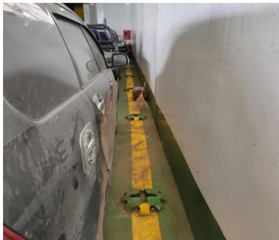
Gambar 4.21 Jarak Sisi Kendaraan Ke Dinding Kapal
