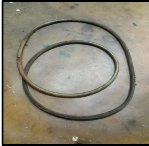
Gambar 4.7 O-ring jacket cover
