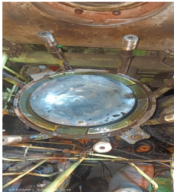
Lampiran 6 Proses overhaul main engine cylinder no.1
