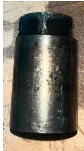
Gambar 2.8 *Retaining nut*
