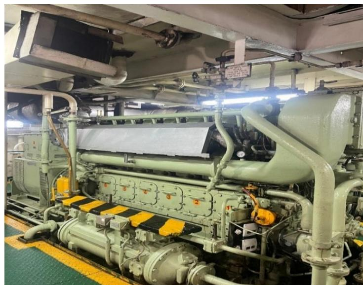
Gambar 2.1 Penampang Diesel Generator Daihatsu 6DL-19(Dari samping)
