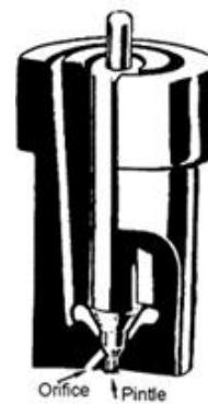
Gambar 2.12 *Injector nozzle* jenis *Throttle* (*Throttle Type*)
