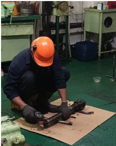
Gambar 4.2 Proses perawatan injector
