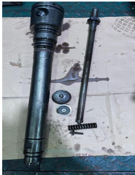
Gambar 4.2 Proses perawatan injector
