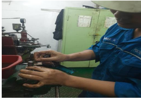
Gambar 4.21 Perawatan Nozzle Injector
