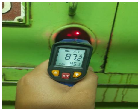
Gambar 4.16 Mesin Diesel Generator Over Heat
