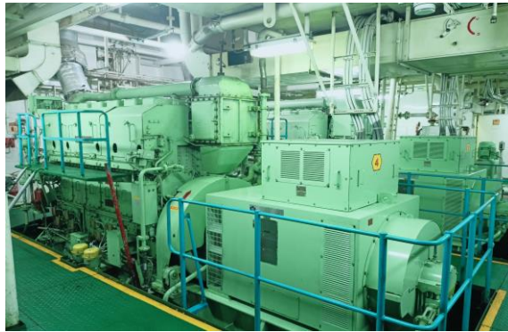
Gambar 4. 2 Mesin Diesel Generator Daihatsu 6DL 24
