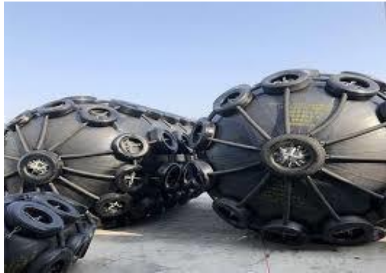
Gambar 2. 11 Fender tipe pneumatic sumber: http://therubbercompany.com
