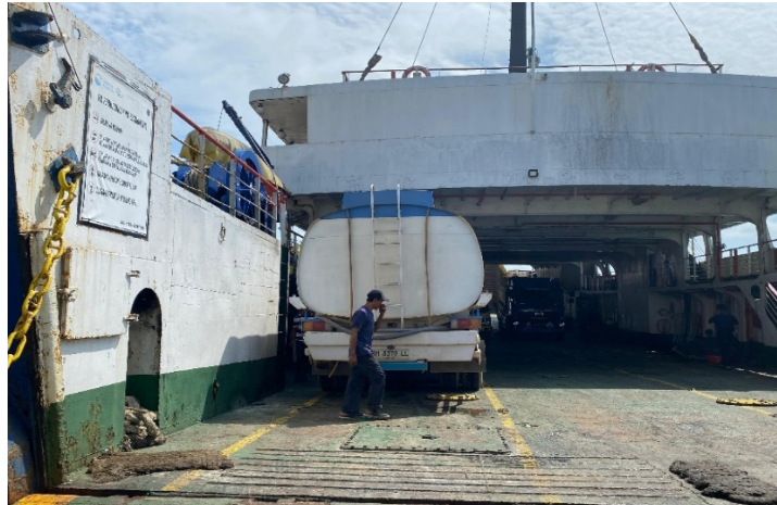
Gambar 4. 39 Proses Pengisian Air Tawar Kapal
